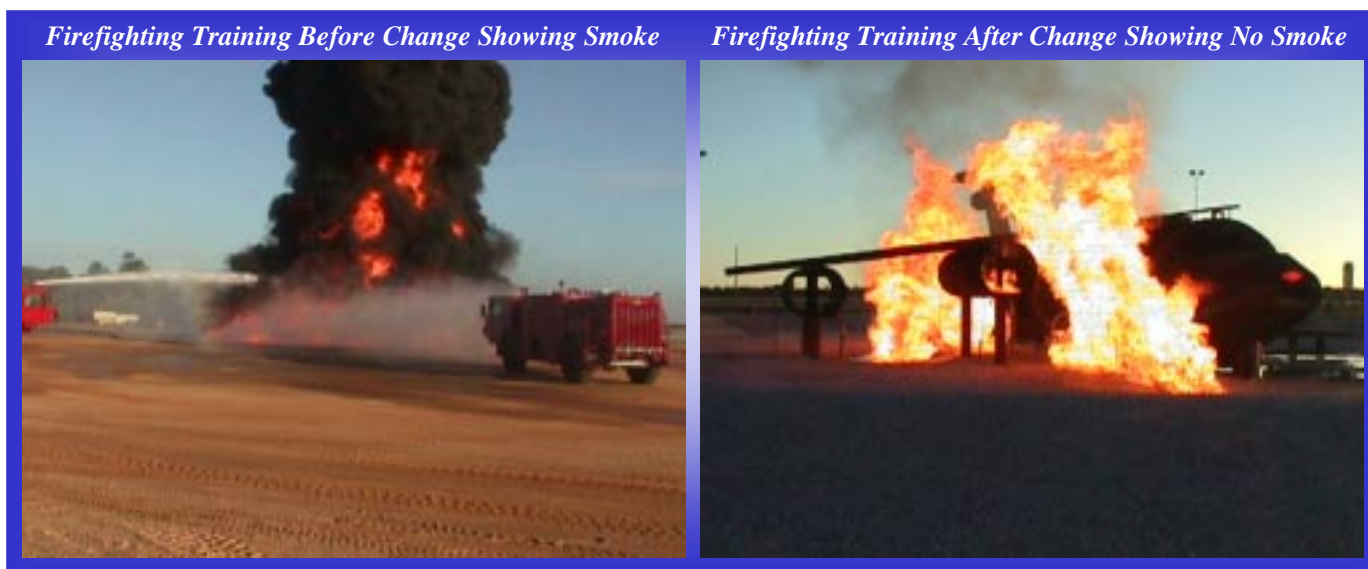
Switching from JP-8 to Liquid Propane Significantly Reduced Smoke Emitted During Firefighting Training as Shown During a Pretest Last Winter at Eglin AFB
