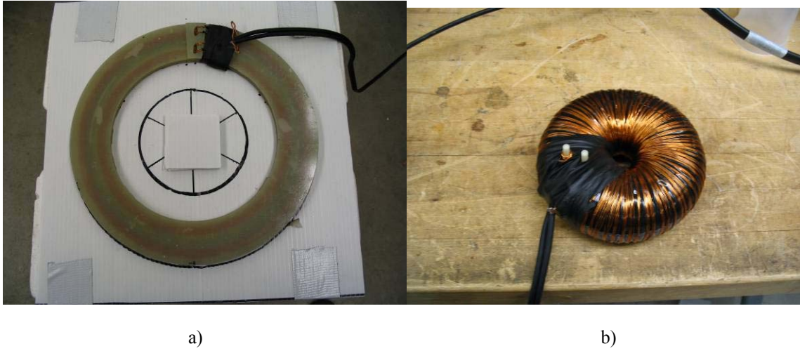
Figure 9. a) Head transformer and b) toroidal bucking transformer for prototype #2. used to measure the transfer function of the system, and two SR560s were used as preamplifiers to amplify the signals V_H and V_B - V_H .
