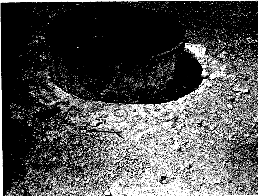
Figure 2.1 (Continued) (g) Close-up of internal surface of casing after Shot 6, 15 lb. (h) External view after shot showing bond between grout and casing.
