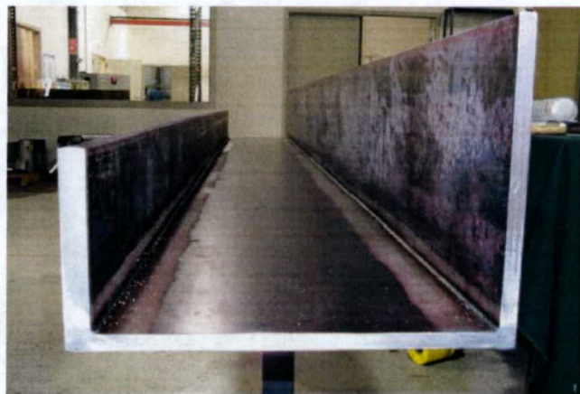
Figure 12.9 – Laser Welded C-section for Test Tank
