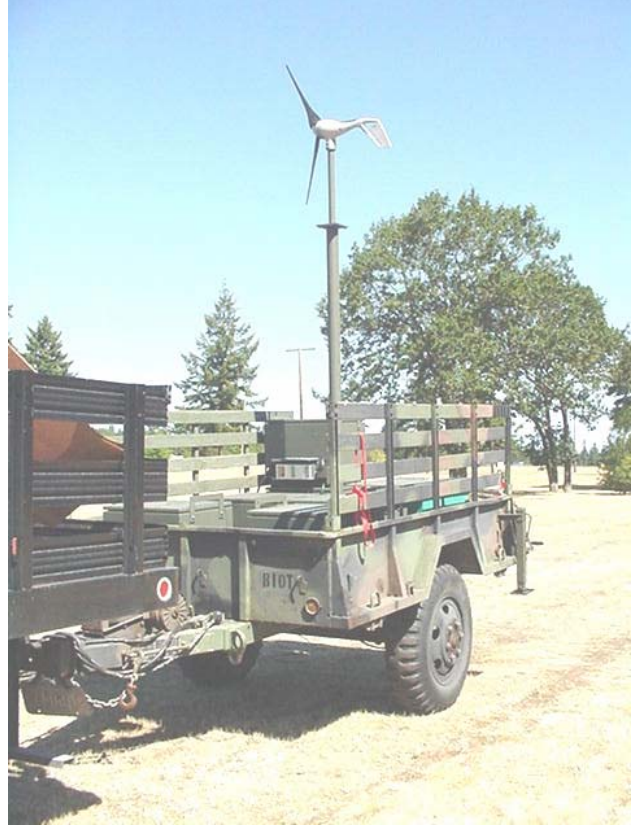
Figure 8 Deployed TACS Power Center
