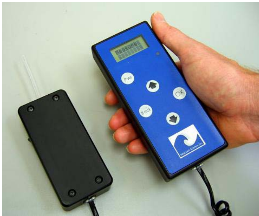
Figure 38. Seacoast Science Prototype Hypergolic Chemical Detector Detector.
