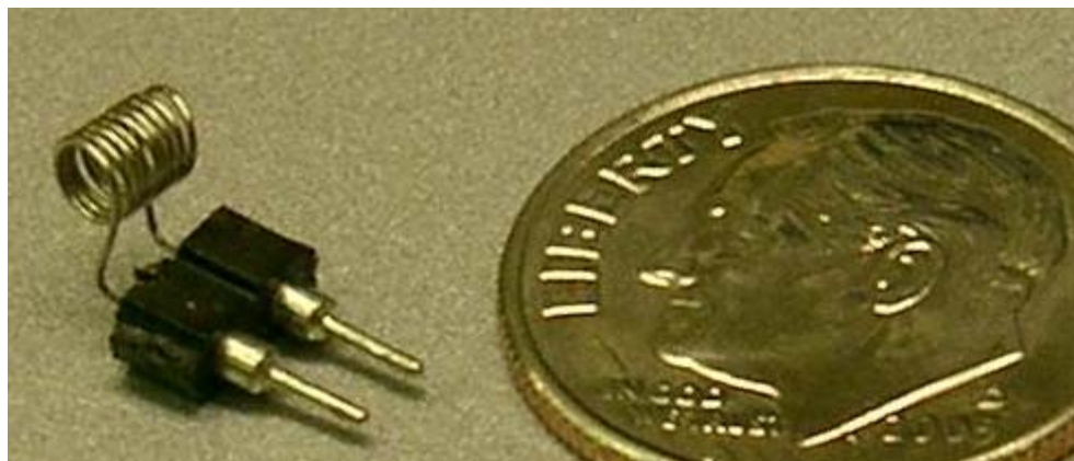
Figure 36. Heated Sensor Element Coated With A Chemoselective Material Coating HC.
