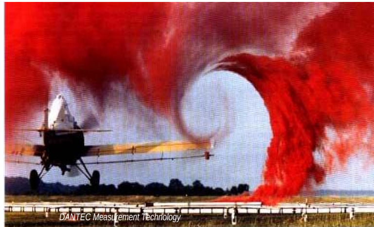
Figure 4.2: Wing Tip Vortex (Picture from DANTEC Measurement Technology)
