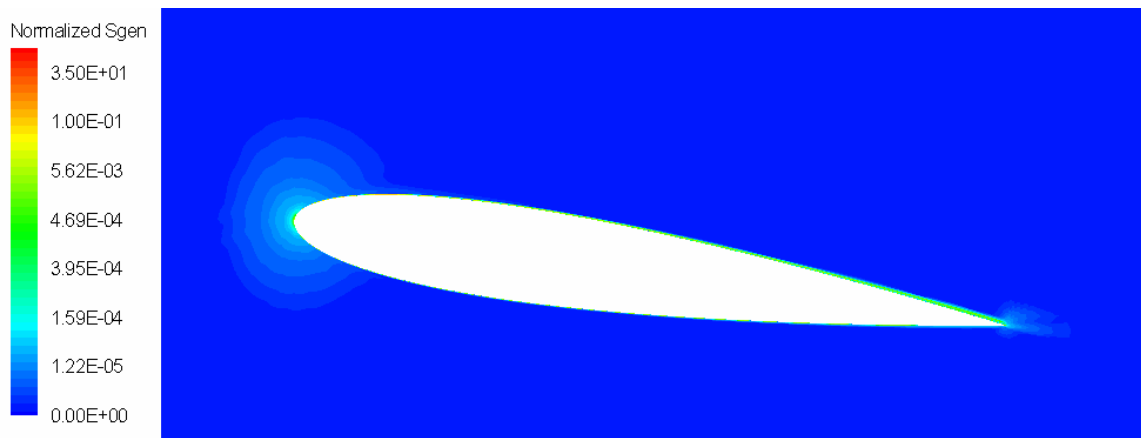
Figure 6.11: Total entropy generation rate for parabolic case at z = 0.5\text{m}
