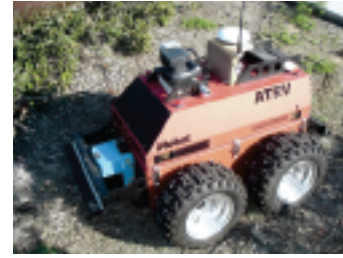
FIGURE 7. Exterior transition platform, iRobot ATRV.
