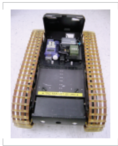
FIGURE 3. Chemical payload package on the MPRS URBOT.
