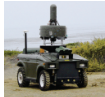
FIGURE 8. MDARS-E vehicle with launch fixture for the 29-inch iStar OAV.
