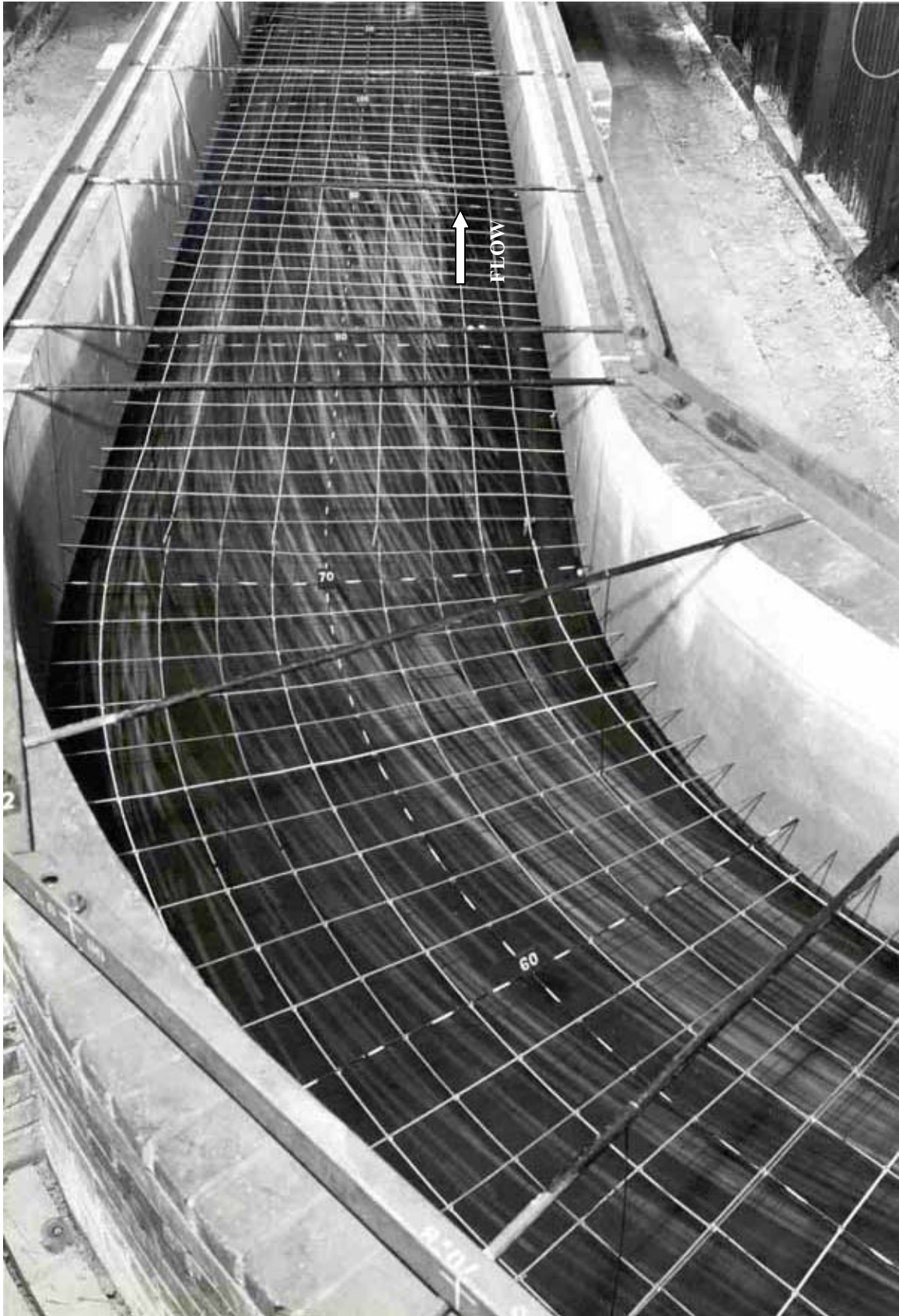
Photo 6. Surface current directions downstream from bend, 2 distortion
