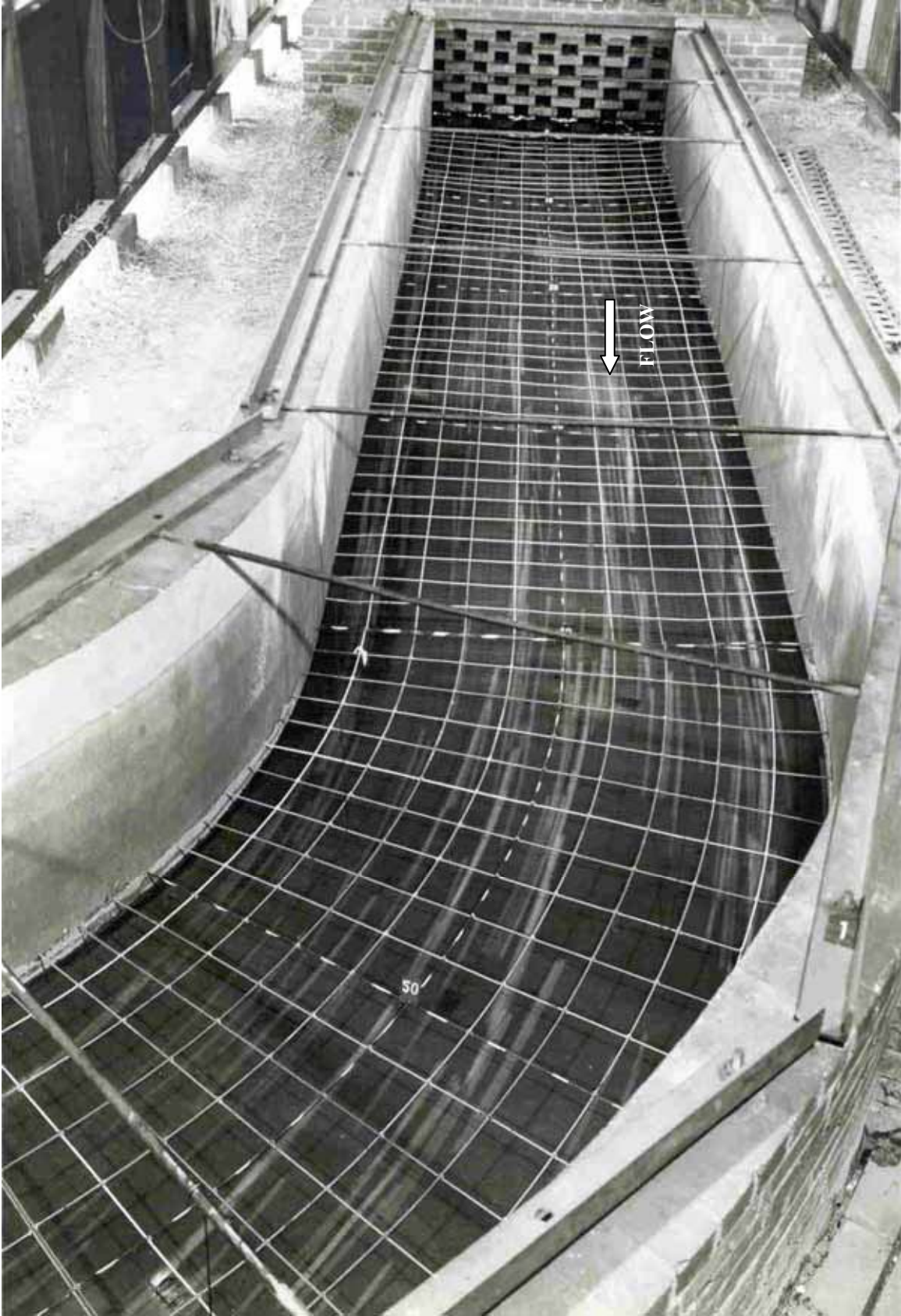
Photo 1. Surface current directions upstream from bend, 0 distortion
