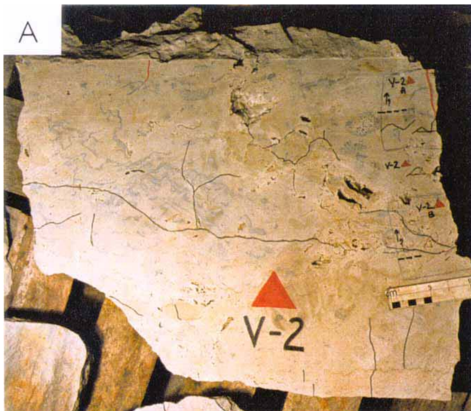
Figure 62. Valders Quarry Test Block V-2-FT sample locations. Arrows show direction perpendicular to interpreted bedding planes based on clay seams and associated stylolites (after Agar 1998)
