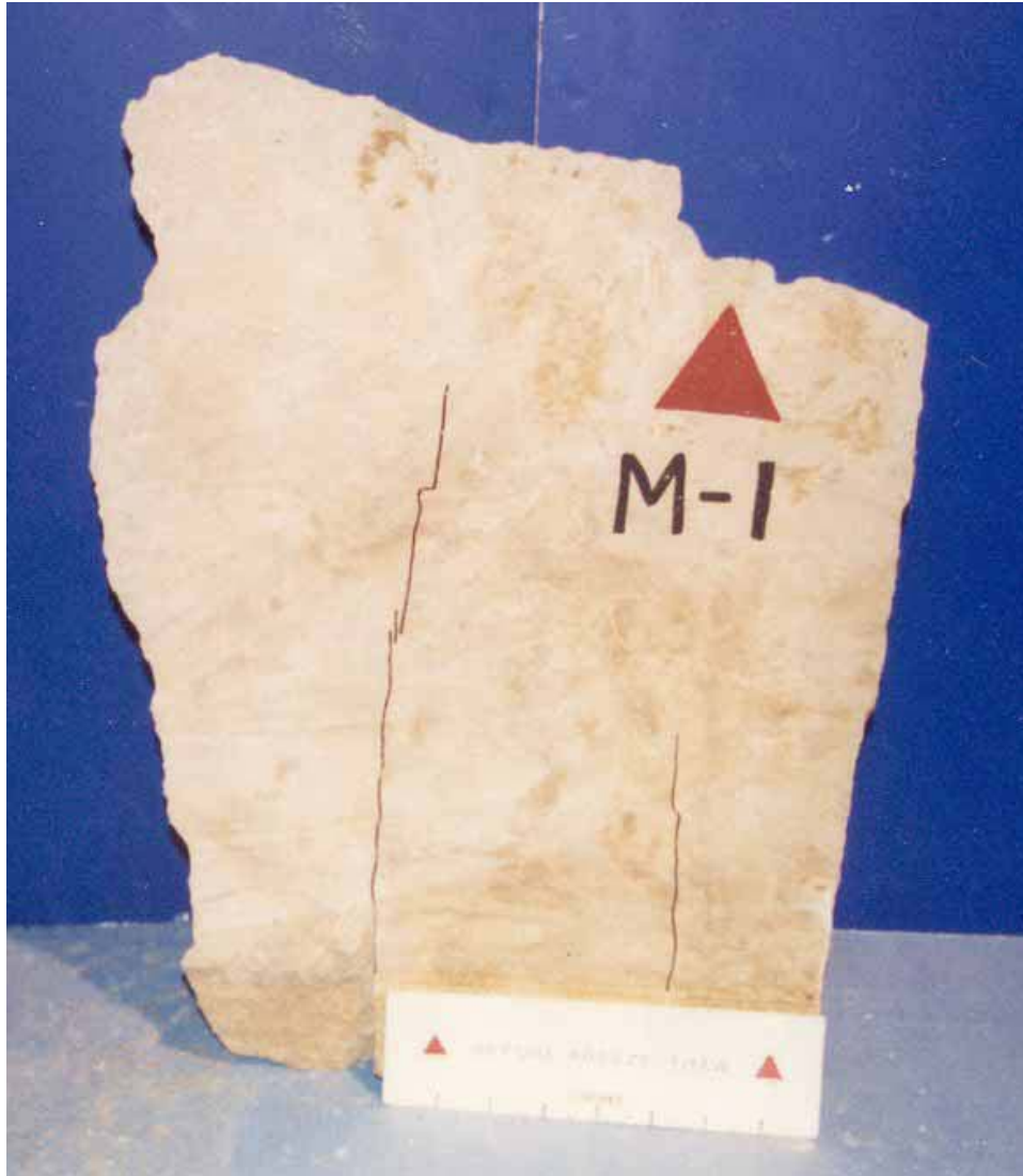
Figure 46. Marblehead Quarry Columbus formation dolomitic limestone accelerated weathering durability Test Block M-1-FT
