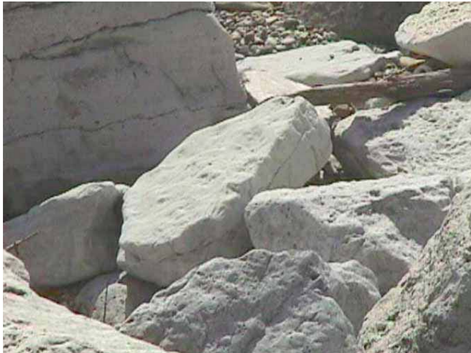
Figure A3. Dolomite armorstones showing stylolites in various degrees of separation
