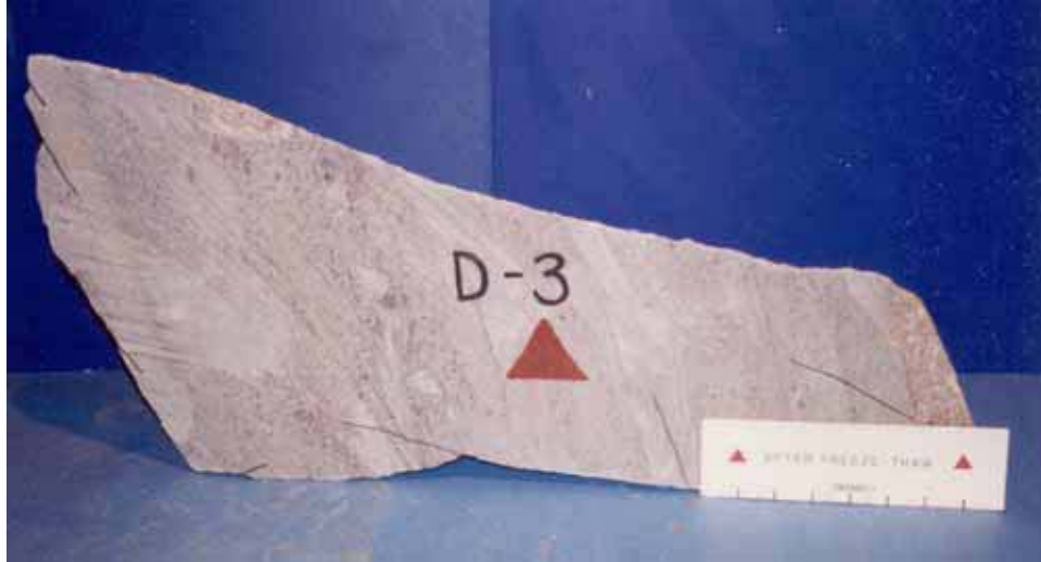
Figure 43. Dempsey Quarry Waterloo formation quartzite accelerated weathering durability Test Block D-3-FT
