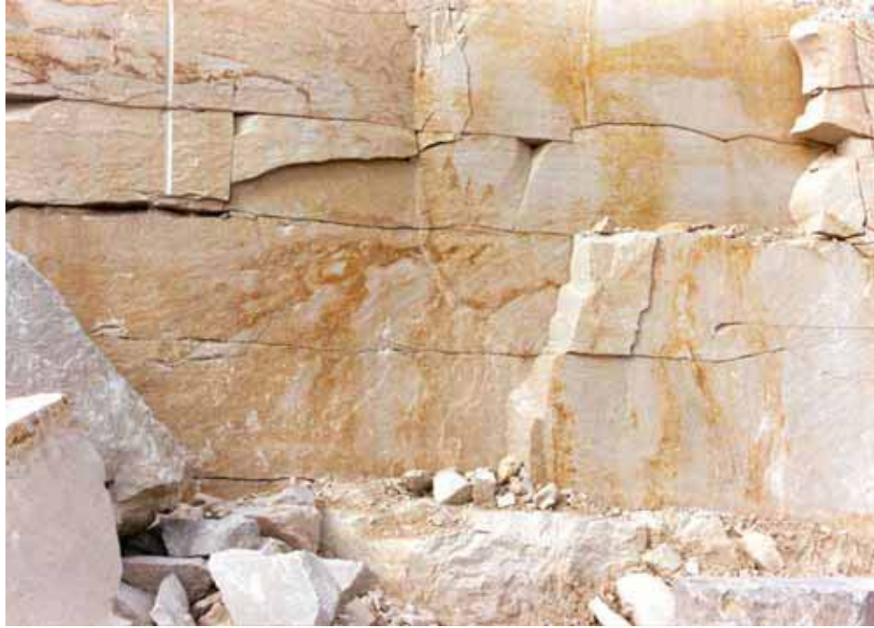
Figure 15. Valders Quarry, Valders, WI, lower bench showing discontinuous horizontal unloading features (after Rock Products Consultants 1995)
