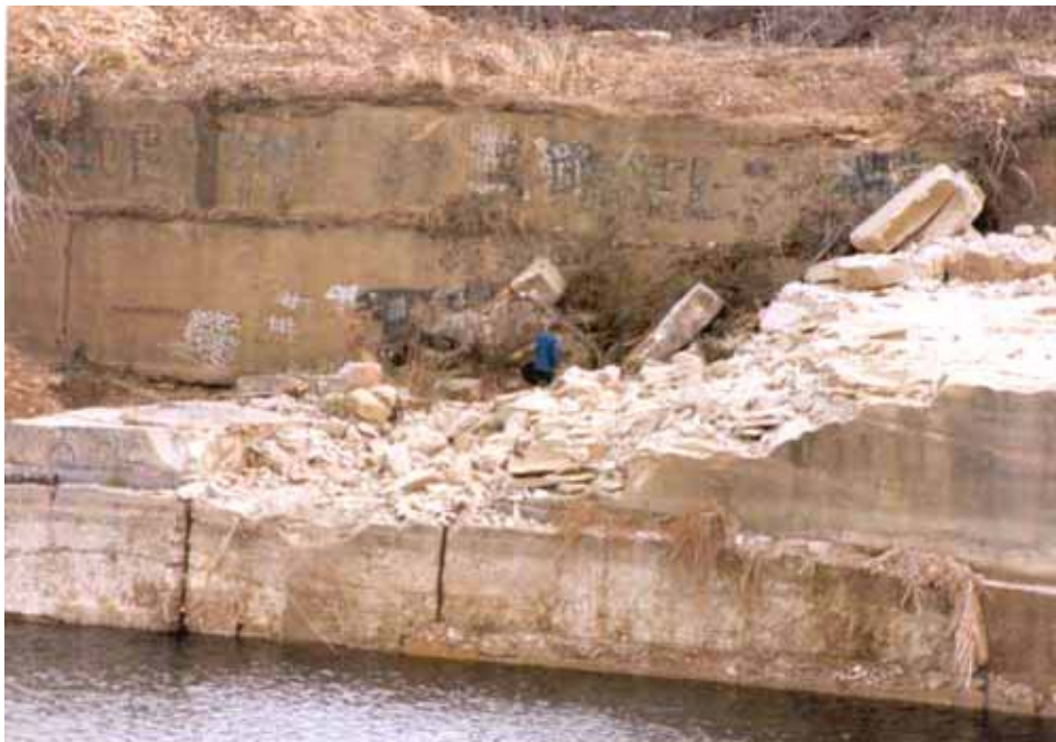
Figure 28. Johnson Quarry, Kipton, OH, area where an attempt was made to produce sandstone blocks by blasting (after Rock Products Consultants 1995)
