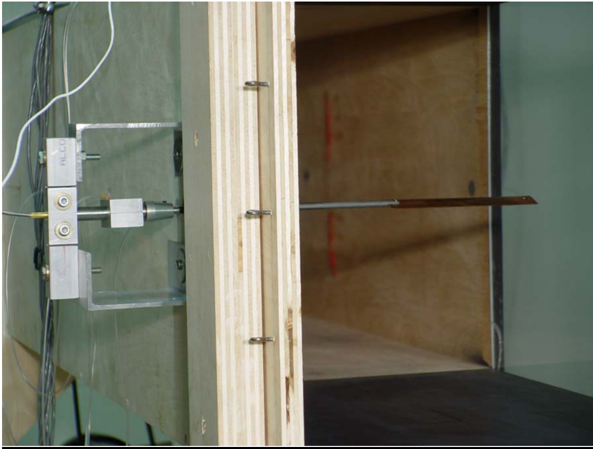
Figure 4.32 Load cell/airfoil configuration
