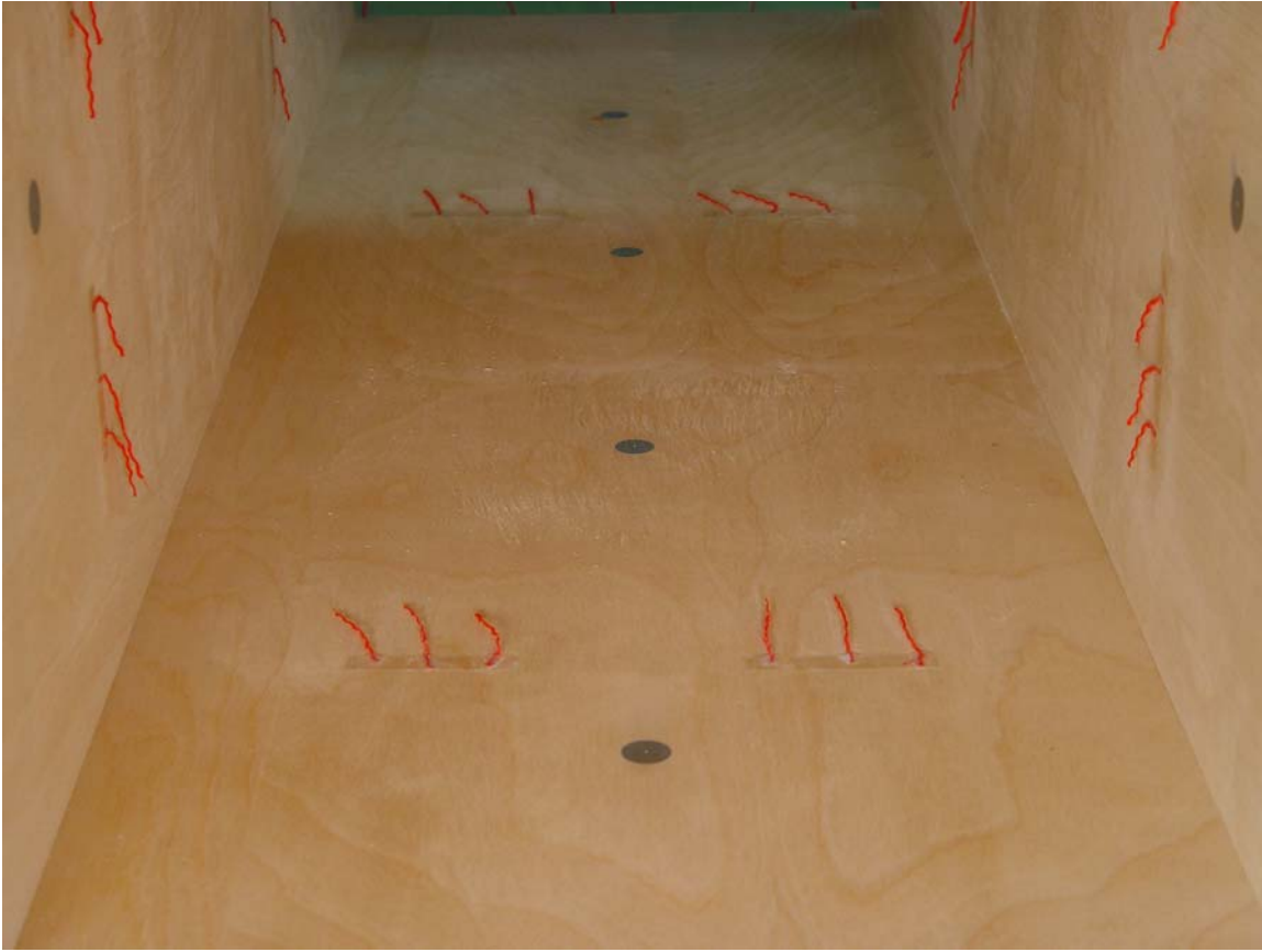
Figure 4.11. View from forward end of the tunnel showing axial ports and part of the forward ring (red strings are tufts)
