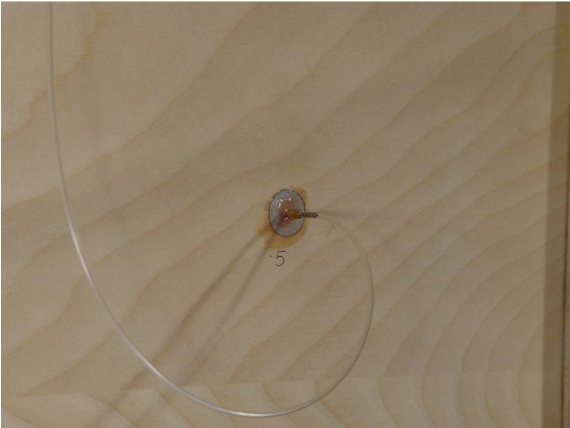
Figure 4.10. Exterior view of a static pressure port plumbed to a transducer
