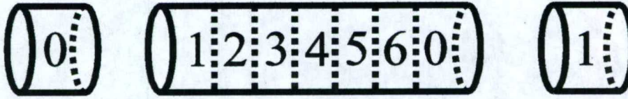
Fig. 1.2: Part of the row of nanotubes with two cuts. Dotted lines in the nanotubes correspond to cuts of the neighboring nanotubes. The regions between them are considered to be ballistic.
