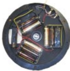
Figure 9: The battery holders embedded into the base of the omnidirectional camera. The omnicam was held "upside-down" while taking this picture.
