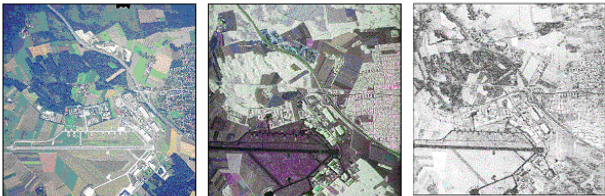
Fig. 14: Optical image (left), polarimetric color coded image (center) and interferometric coherence (right) over Oberpfaffenhofen (Germany)
