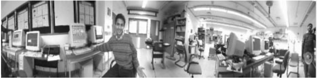
Figure 14: Panoramic video stream generated using the polycamera shown in Figure 11. The panorama is computed using a look-up table, which is constructed taking into account the relative orientations of the four wide-angle cameras as well as their distortion parameters.
