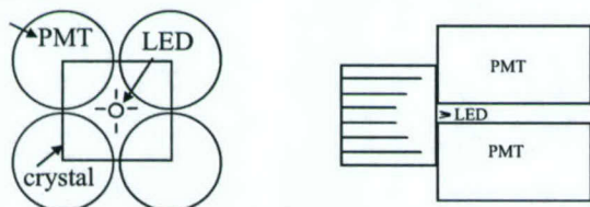
Fig. 1: An LED at the center of a cluster of PMTs is used to tune a scintillation detector regardless of the temperature sensitivity of its light output.
