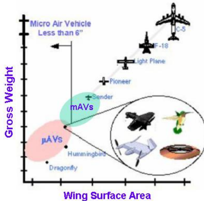
Figure 2.4 The MAV compared to existing flight vehicles extracted from [32:3]
