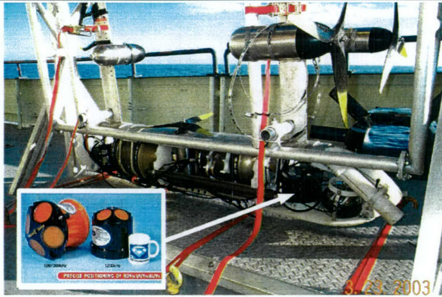
Figure 1-16 A RD Instruments 1200 kHz Workhorse Navigator DVL is shown in-situ on the bottom hull of the SeaBED AUV (outer hydrodynamic shell removed).
