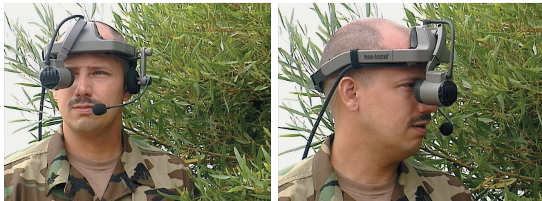
FIGURE 1. Based on a commercial wearable computing system and augmented with SSC San Diego-developed software and display concepts, AITS is used for field surveillance and monitoring. With use of see-through display components and head-tracking technology, symbology can appear superimposed over the environment.
