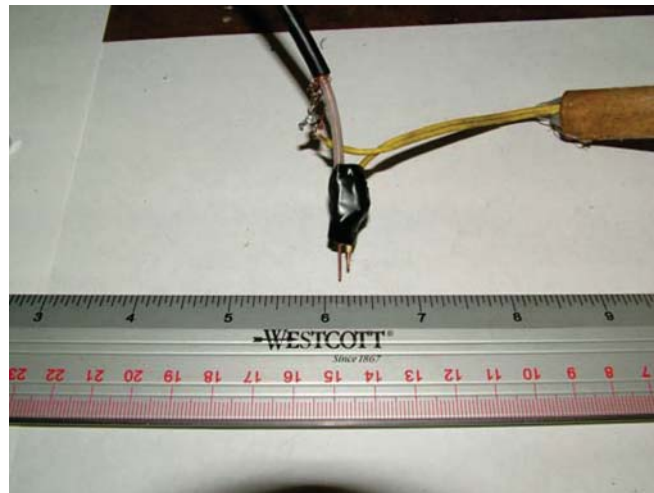
Fig. 3 — Field rigged spark gap between the radiating antenna and pulse-forming line
