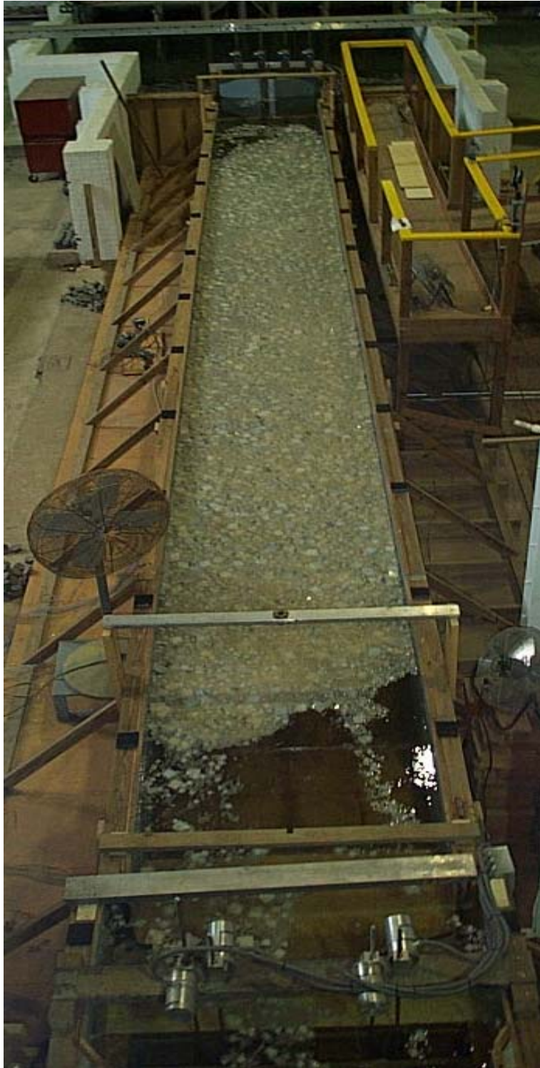
Figure 7. Test drawing ice from upstream approach into lock chamber viewed from upstream
