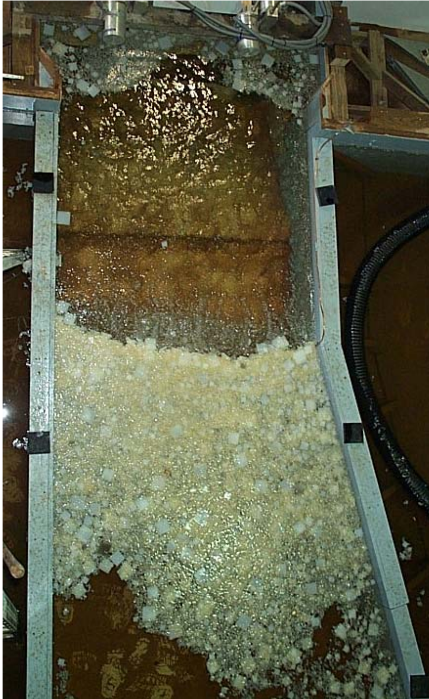
Figure 18. High-flow air curtain retaining upper approach ice during lock filling
