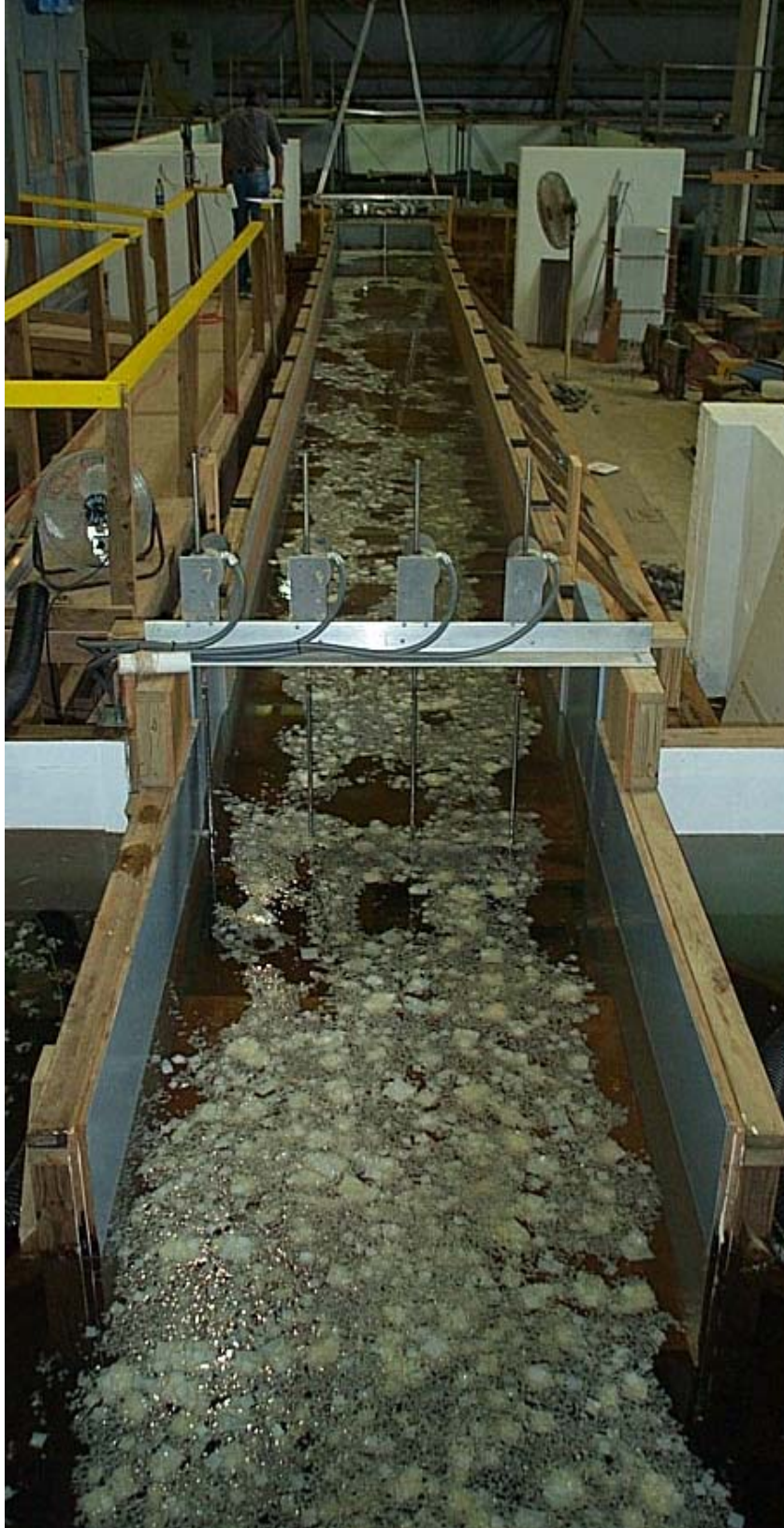
Figure 8. Test flushing ice from lock chamber viewed from downstream
