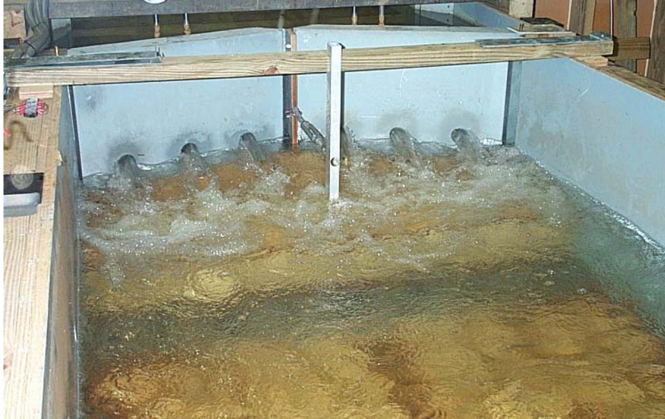
Figure 13. Manifolds in upper miter gates to create surface currents for ice flushing
