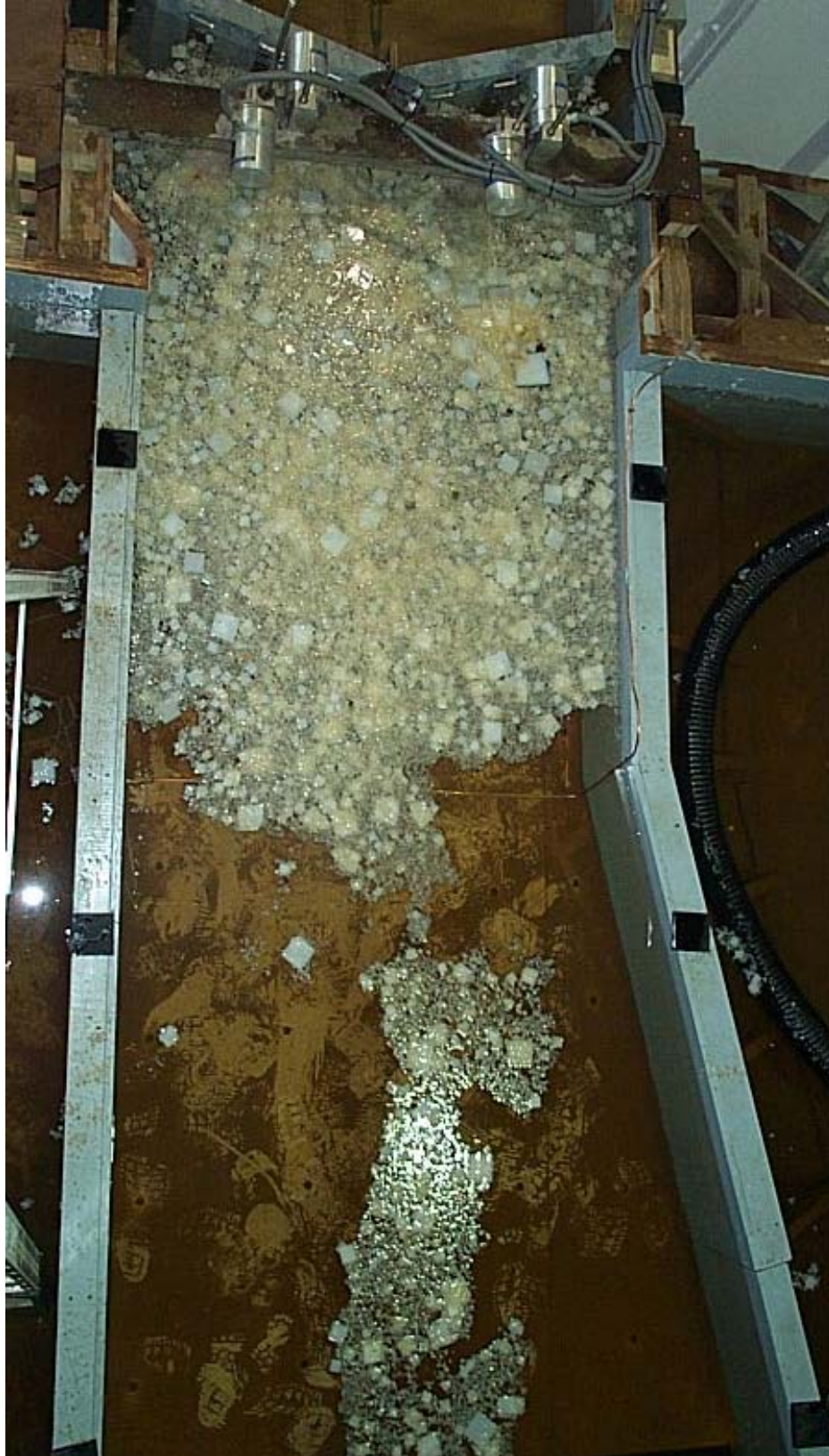
Figure 9. Upper approach ice accumulation test
