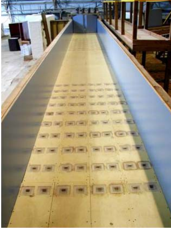
d. Ports inside lock chamber Figure 3. (Sheet 4 of 9)
