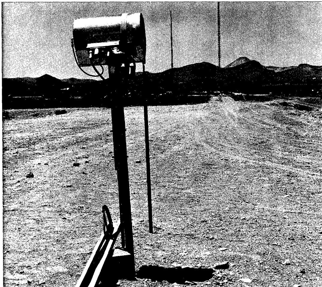
Fig. 2.4—Normalizing Channel No. 1—detector, mount, and preamplifier. BREN tower can be seen in background.
