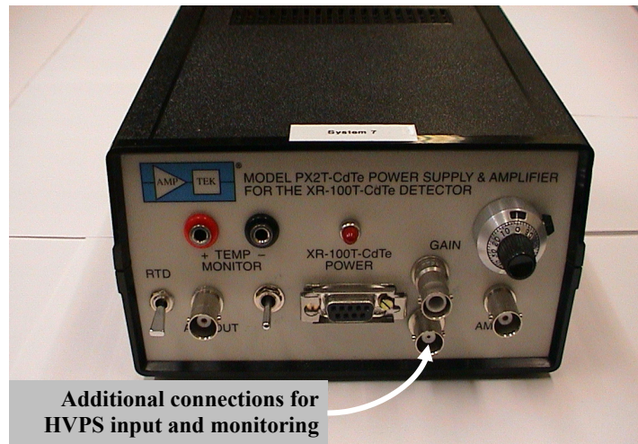
Figure 23. Modified PX2T for external power supply.
