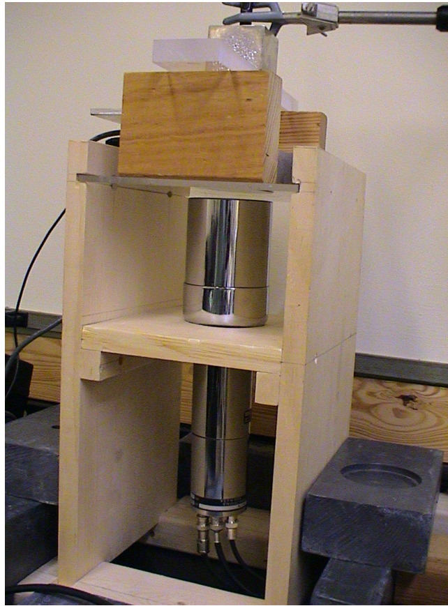
Figure 26. Compton spectrometer housing
