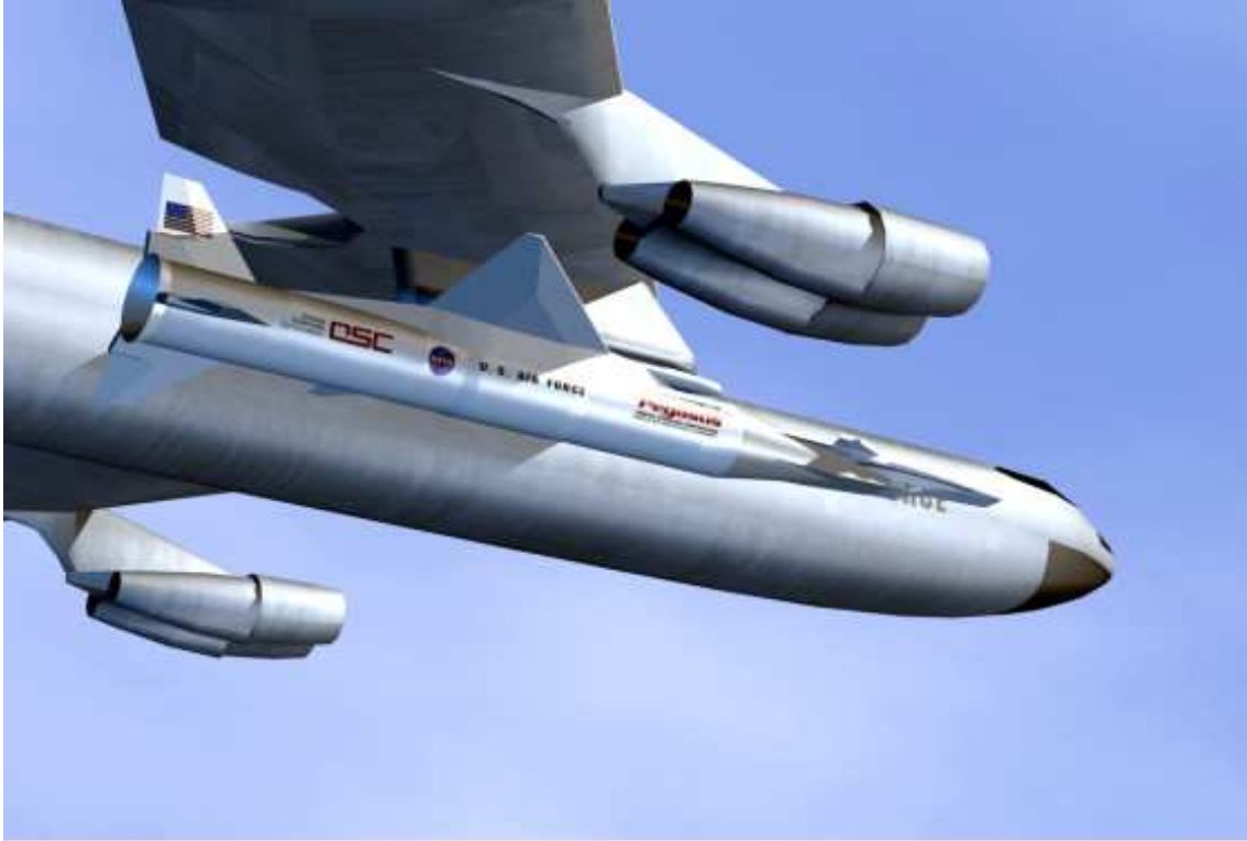
Dryden Flight Research Center ED97 43968-04 B-52 CARRY-ALL: This artist's concept depicts the Hyper-X research vehicle riding on a booster rocket prior to being launched by Dryden Flight Research Center's B-52 at about 40,000 feet.
