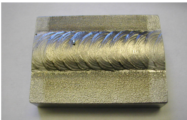
Figure 2. Monel/304L welds made using GTAW. High heat input welds with argon shielding gas exhibited surface “slagging” and solidification cracking (above). The use of 95Ar-5H 2 shielding gas produced good quality welds (left).
