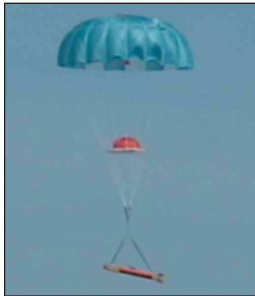
Fig. 7 — Vehicle descending with the parachute deployed
