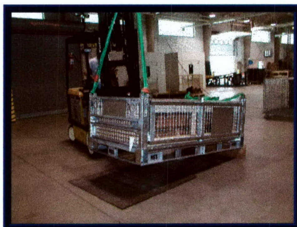
Photo 3. Example of Edgewise Rotational Drop Test (MSTF Low)
