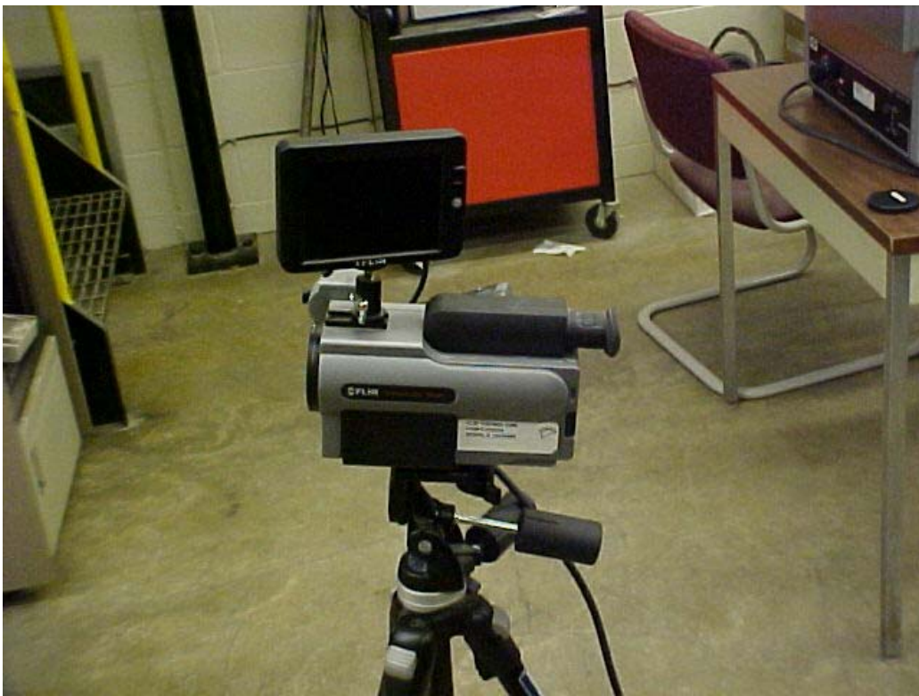
Figure 13. FLIR IR Camera
