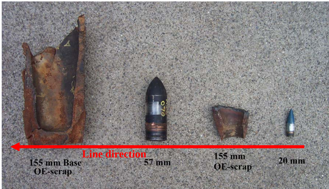
Figure 37. Measurements over each of the two UXO (57 mm and 20 mm projectiles) and 2 IROS (155 mm base and 155 mm nose section) targets were made with each target positioned at the center of the platform, “primary axis” perpendicular to the line direction (shown in red). The orientation of each item, reflects its orientation relative to the collection direction during surveying: the upper end of each item (“nose”), as shown in the figure, pointed towards increasing line number. Five planes, at varying multiples of the body-length, were collected above each target.
