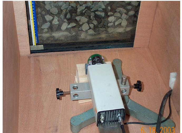
Figure 4. Side view of flume and laser doppler used in experiments of B. Hofland (Delft University of Technology, The Netherlands, written commun., 2001).
