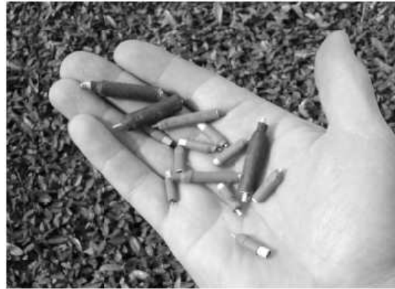
Figure 2. Coaxial solid-state microthrusters 1/8”-1/4” in diameter ready for testing.
