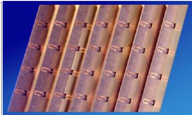
Figure 7. Planar Array Test Article
