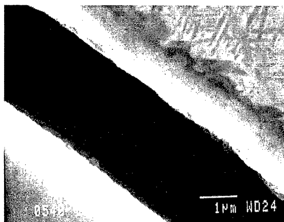
Figure 2-17 Micrograph of carbon layer after thermal exposure at 650 °C for 100 hours
