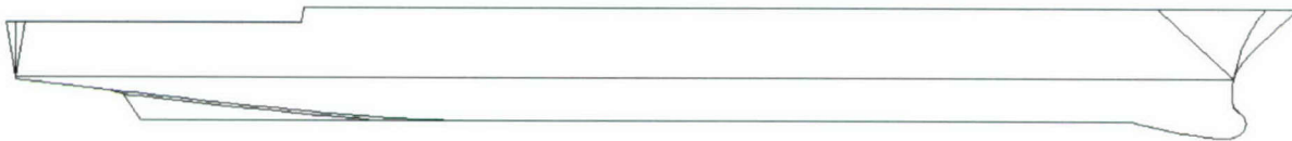
Figure 2. Composite of Profiles for Flare, Wall-Sided, and Tumblehome Hulls
