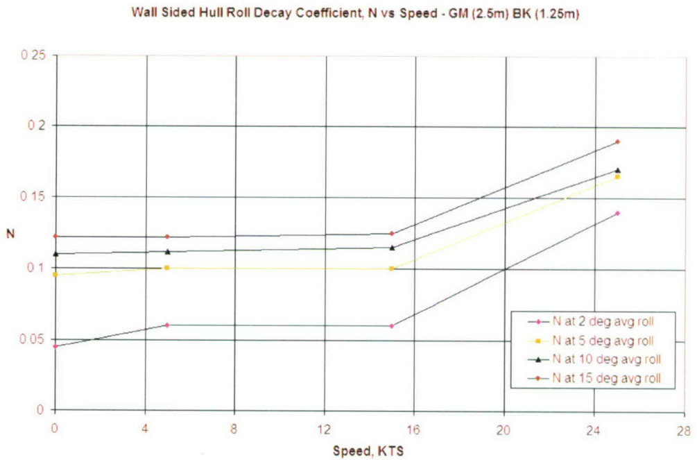
Figure 74. Wall Sided Hull Roll Decay Coefficient versus Speed for GM=2.5m and BK=1.25m.
