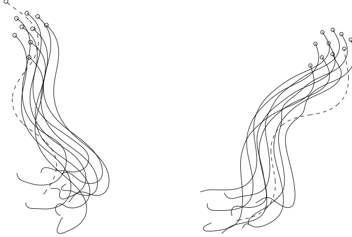
Fig. 11. Formation initialization for ten vehicles, one of which (dashed) follows a prescribed steering program unaffected by the other vehicles (for two different sets of random initial conditions).
