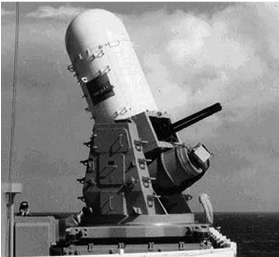
Figure 37. Vulcan Phalanx. The Navy fitted a number of its ships with the fast-firing Vulcan Phalanx for close-in protection against aircraft. (Reprinted from http://www.bb62museum.org/images/phalanx.jpg .)
