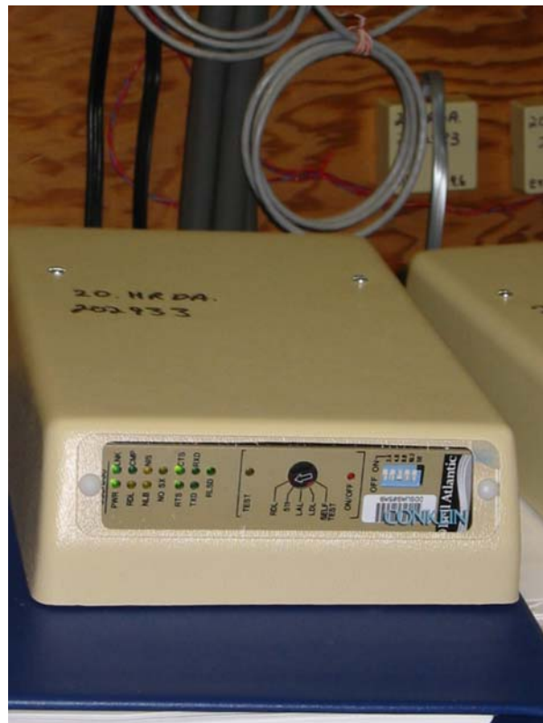
Figure C-17. CSU/DSU (Data Circuit interface).
