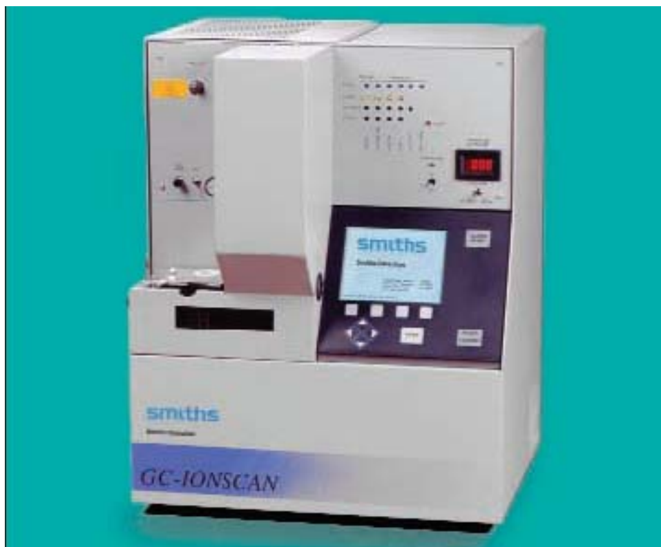
Figure 9. The GC-IONSCAN™ portable ion mobility spectrometer . Photo used with permission. http://194.105.117.18/Documents/LifeSciences/GCIonScan_LS.pdf
