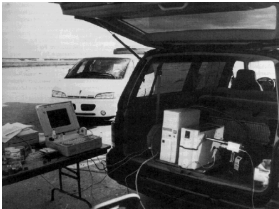
Figure 7. A vehicle-based DSITMS system ( http://apps.em.doe.gov/ost/pubs/itsrs/itsr69.pdf )
