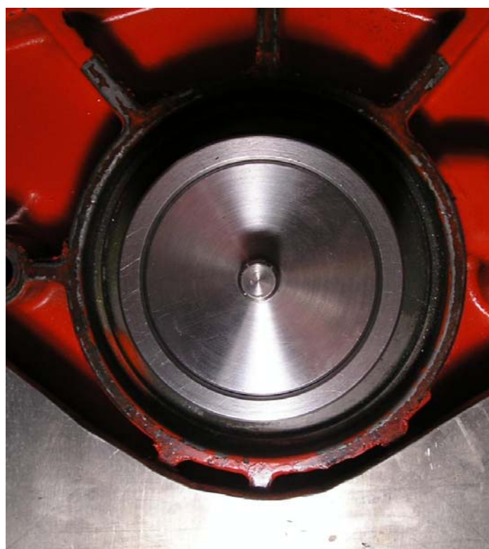
Figure 9. Encoder mount with collar installed after filing.
