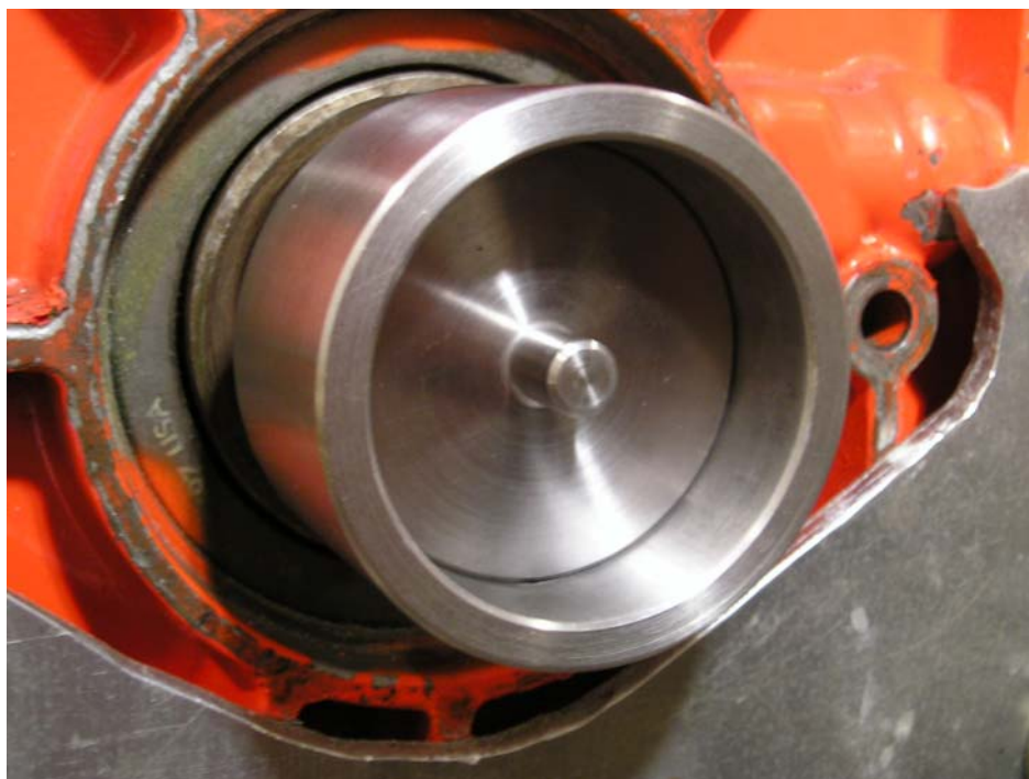
Figure 8. Installation of the collar over the encoder mount before the set screws were filed down
