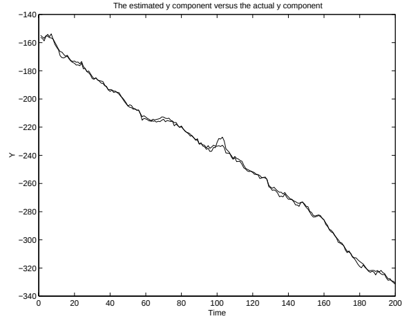
Figure 5: Estimated x_2 component versus the actual x_2 component of the position of the car. At time 100 there is a cycle slip of strength -20 for the measured phase of the carrier from pseudo satellite (1).
