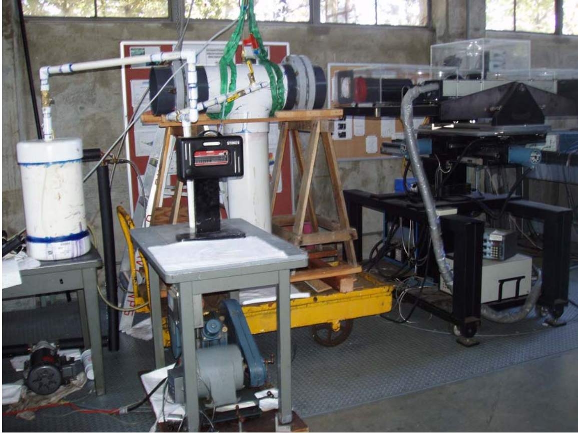
Figure 11. View of LDV system with the vacuum chamber.
