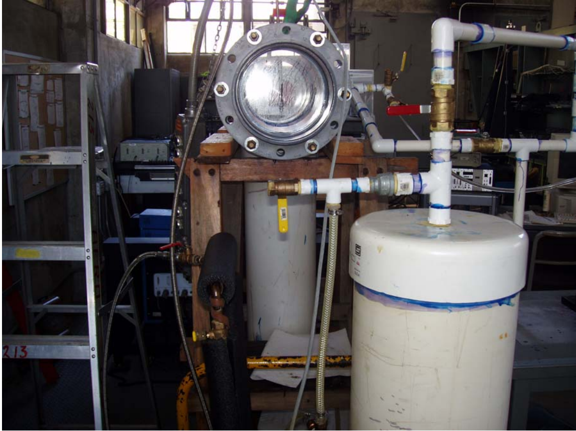
Figure 9. End view of the vacuum chamber showing windows and oil reservoir.
