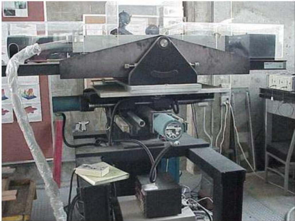
Figure 10. LDV system showing laser and traverse mechanism.
