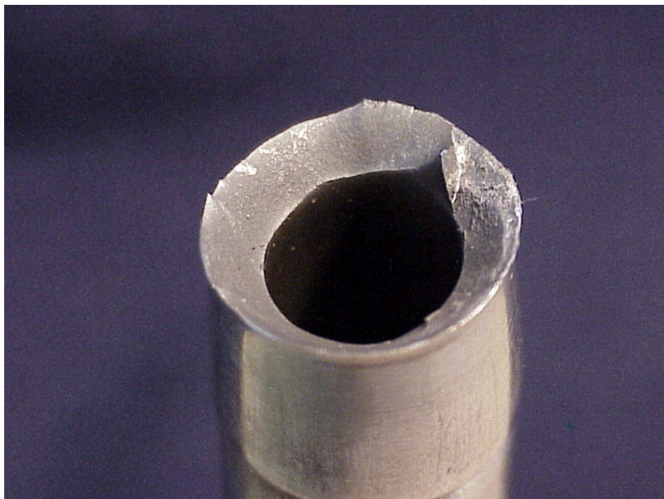
Figure 11. Lower Spindle Fracture Surface
