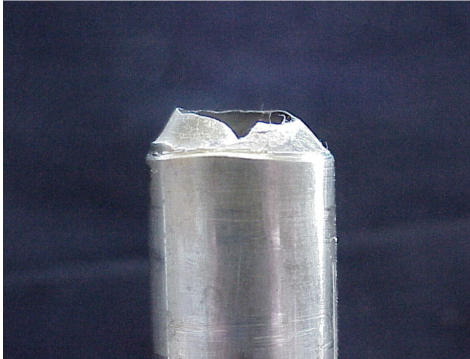
Figure 10. Upper Spindle Fracture Surface (Side View)
