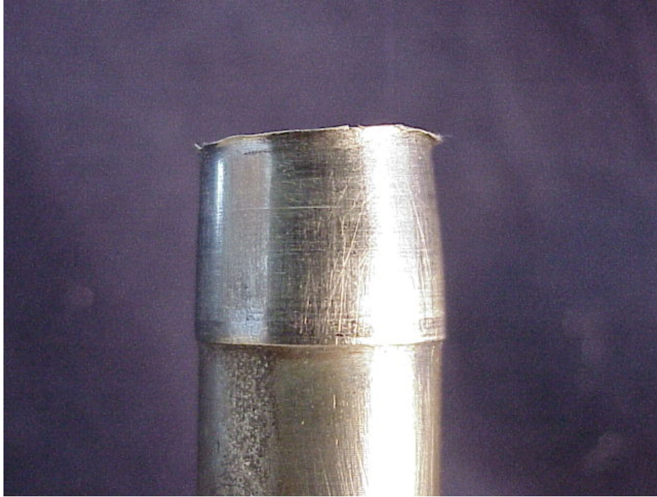
Figure 12. Lower Spindle Fracture Surface (Side View)
