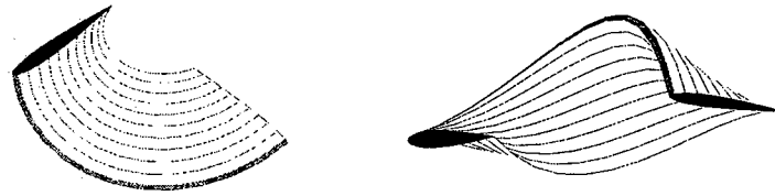
Figure 2.8: Deformations represented by a single element with constant strain distribution.
