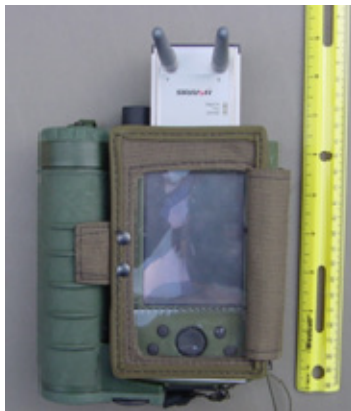
Figure 47. D-DACT with Protective Dome Removed and SecNet-11 Card Inserted
