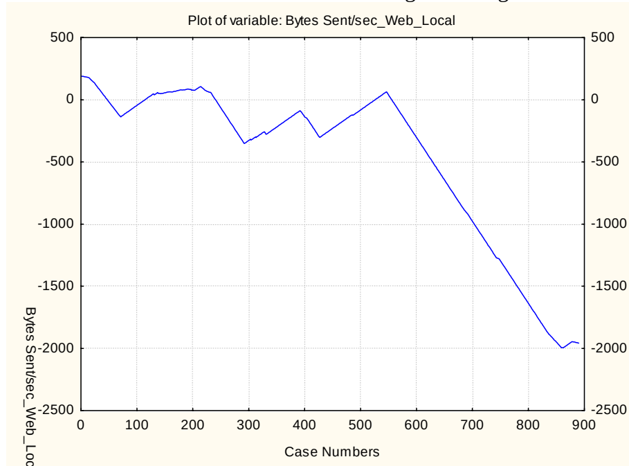
Figure 39. Network Interface(Intel[R] PRO_100 VE Network Connection - Packet Scheduler Miniport)\Bytes Sent/sec, ARP Poison, Web Browsing, Local.
