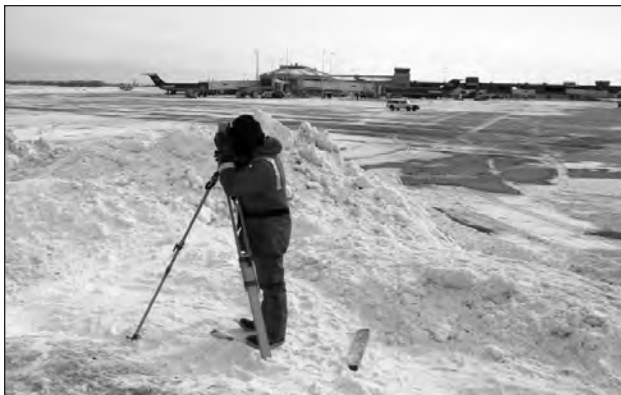
Surveying snowbanks at General Mitchell International Airport for studying aircraft deicers in snow.
