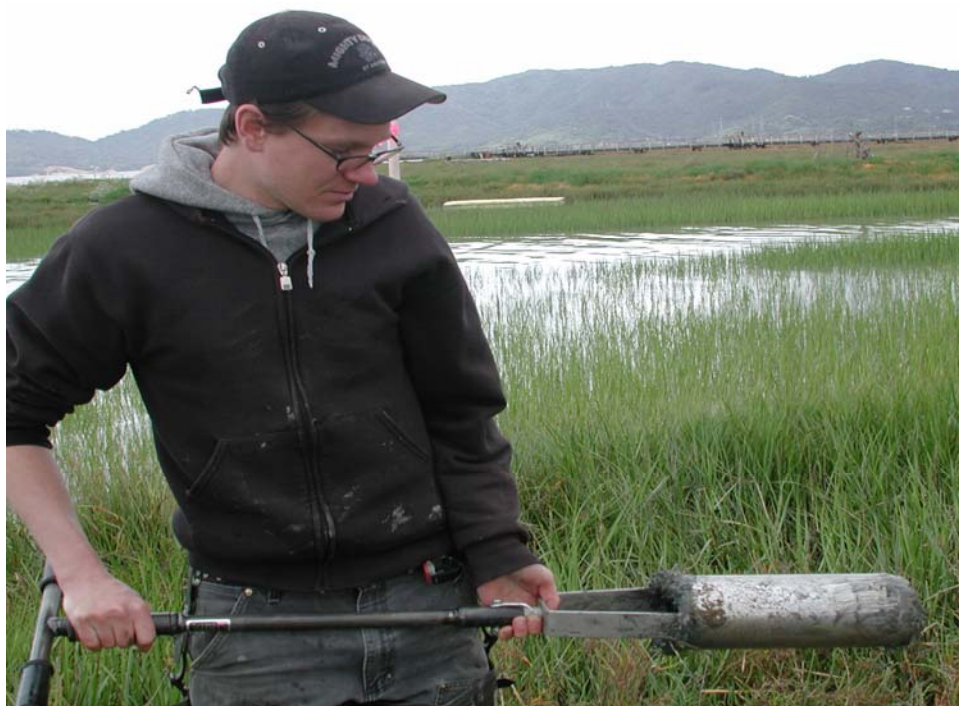
Figure 3-2. Sediment corer constructed to collect 9.5-cm-diam vegetated sediment cores
