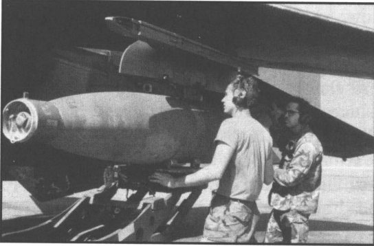
TOP: A GBU-10 laser-guided bomb being loaded onto an F-111 prior to a “tank plinking” mission.
