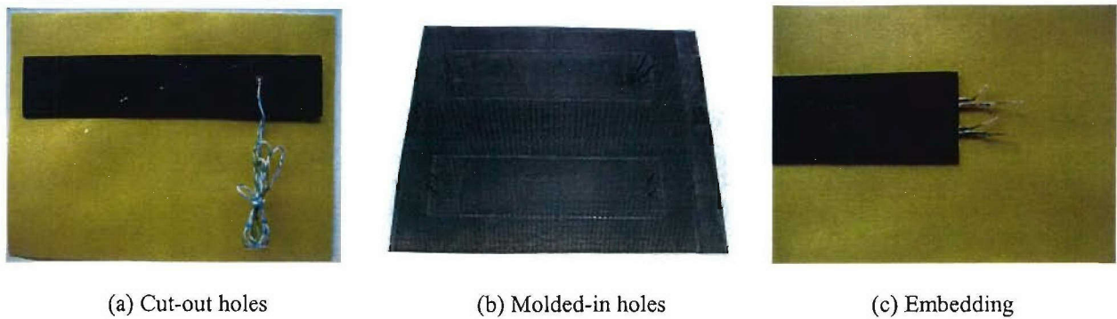
Figure 4.2. Three techniques to take the lead wires out in ACPs with embedded piezo patches.
