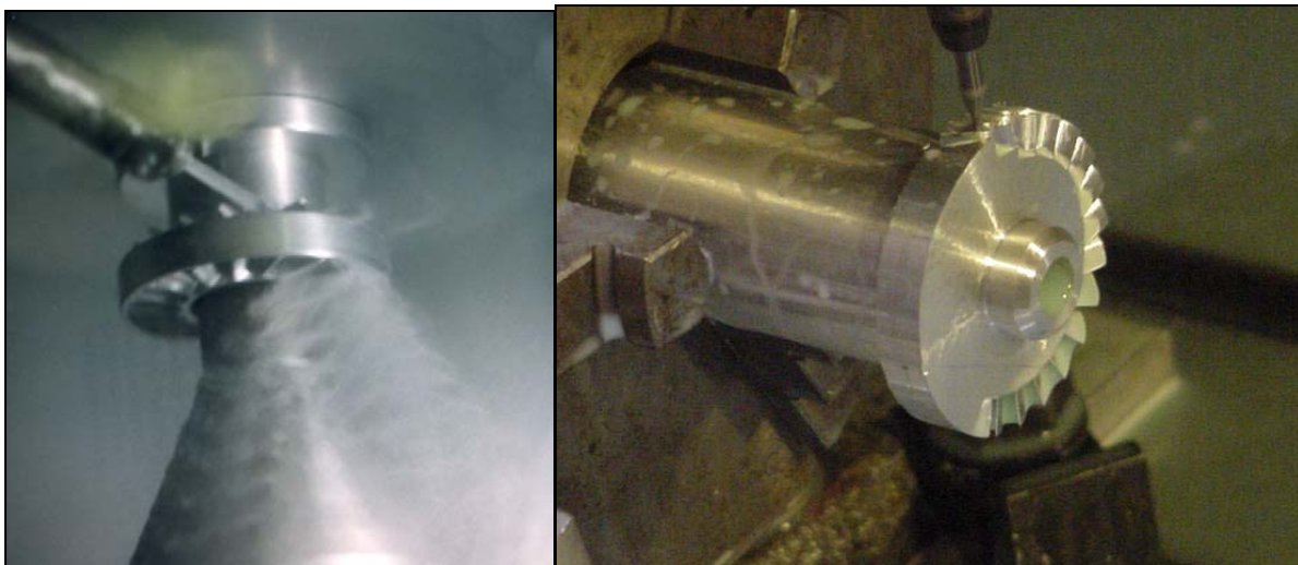
Figure 6: Efficiency Testing and Rapid Prototyping of Turbines at AEI
